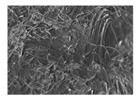
Photo 6: Condition after 100 OTEX washes and drying at 180°F.
