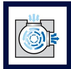
OTEX utilises an oxygen concentrator which takes in air and converts it to 90% pure oxygen
